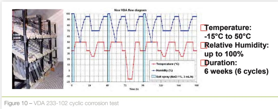
Figure 10 – VDA 233-102 cyclic corrosion test
