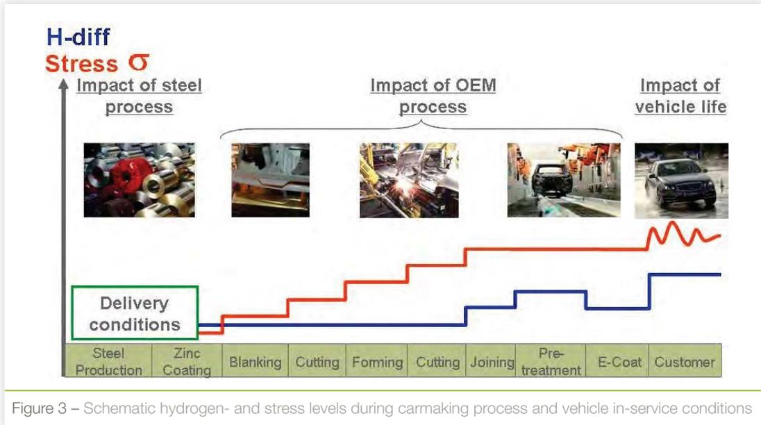
Figure 3 – Schematic hydrogen- and stress levels during carmaking process and vehicle in-service conditions
