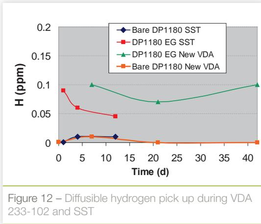
Figure 12 – Diffusible hydrogen pick up during VDA 233-102 and SST
