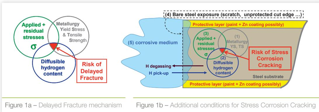
Figure 1a – Delayed Fracture mechanism      Figure 1b – Additional conditions for Stress Corrosion Cracking
