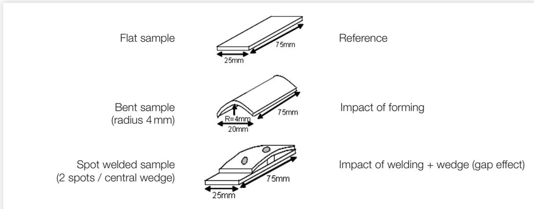
Figure 8 – Specimens for TDA measurements
