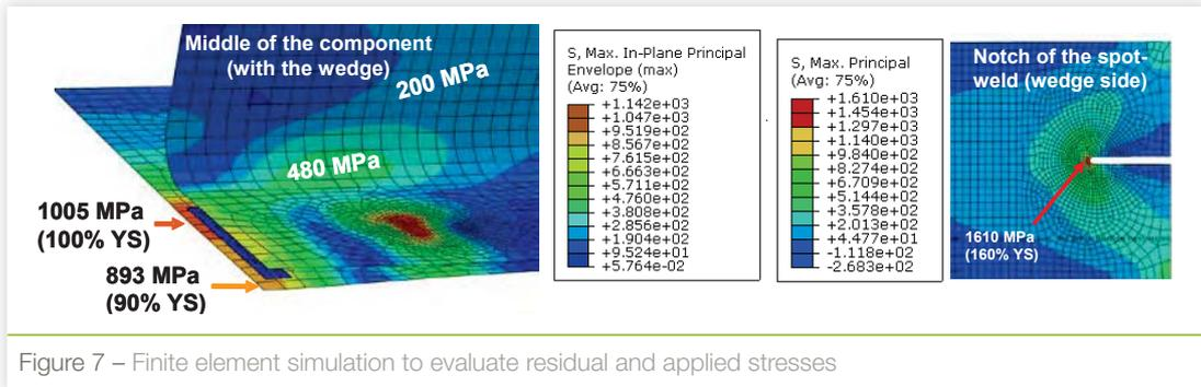
Figure 7 – Finite element simulation to evaluate residual and applied stresses
