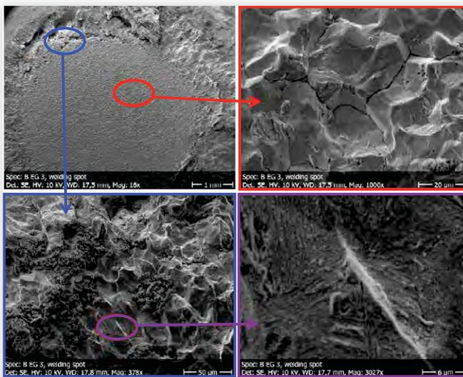
Figure 14 – Fractographic examination of the failed spot-weld
