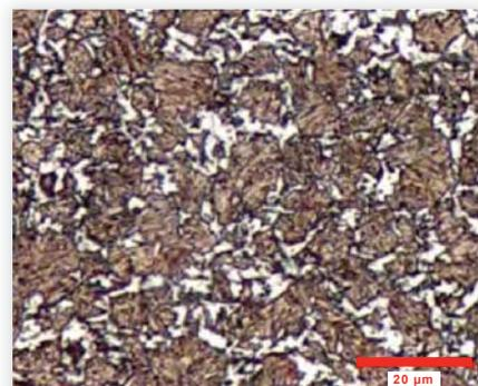
Figure 4 – Microstructure of DP1180 (sodium disulfite etching)
