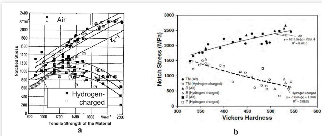
Figure 2a and b – “Crocodile” diagrams starting over 1000MPa Tensile Stress: a from,<sup>3</sup> b from<sup>4</sup>
