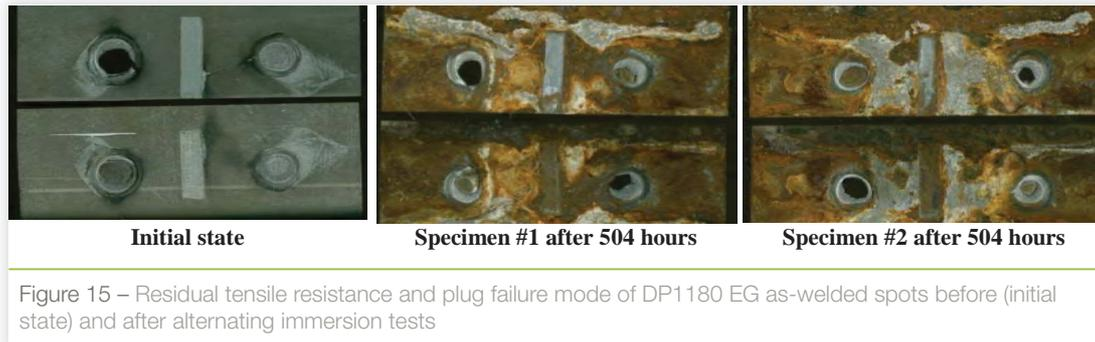
Figure 15 – Residual tensile resistance and plug failure mode of DP1180 EG as-welded spots before (initial state) and after alternating immersion tests
