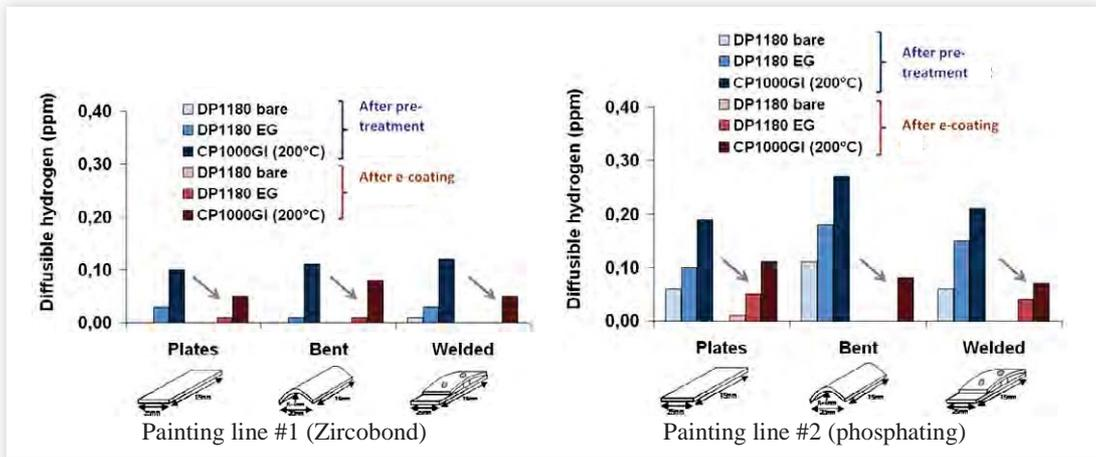
Figure 9 – Hydrogen pick up during e-coating
