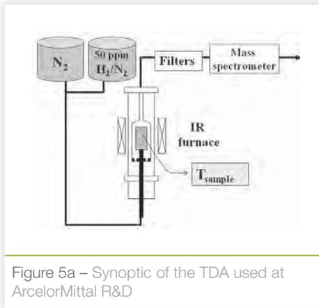
Figure 5a – Synoptic of the TDA used at ArcelorMittal R&D
