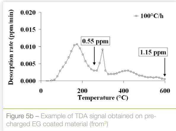
Figure 5b – Example of TDA signal obtained on pre-charged EG coated material (from<sup>3</sup>)
